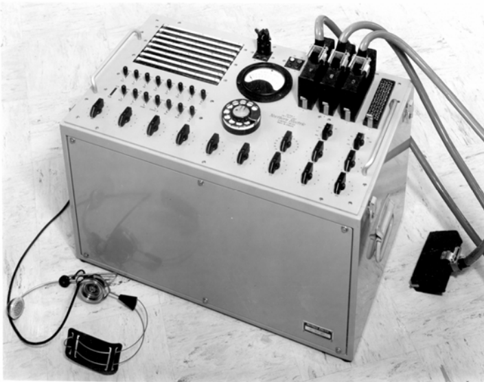
A Northern Electric S.A.-1 Test Unit was used to test the dial lines prior to the installation of the S.A.-1 Community Crossbar Equipment
